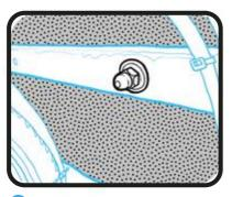
...and the two closed end nuts attach to the front plate.
