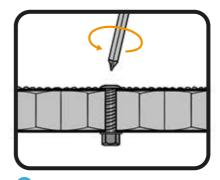
Screw tension should indicate a small dimple on the honeycomb surface.
