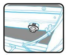
2 The three thread locked nuts lie underneath the bottom plate...
