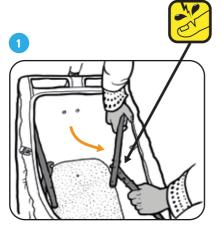
Bend the bars on the roof of the Canopy into position. Be careful -you could cut your fingers!
