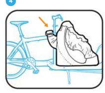
Attach the velcro on the bicycle frame. Remember to screw the two bolts from **Step 1** through both Canopy frame and Bullitt frame.
