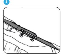
Tighten the screws with Tool 3 (the Hex/Allen Key), and repeat on the opposite side of the Canopy.
